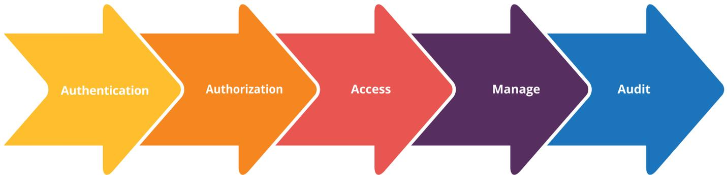
**1. Authentication** - First, a credential is authenticated. After a user presents a credential (mobile credential or car/key fob) at a reader, that credential's data is sent to the Access Control Unit (ACU), where the ACU determines if this credential is known and recognized by the system. If a credential has been added to the system during an Internet outage, the ACU will not recognize the credential until the Internet is restored.
